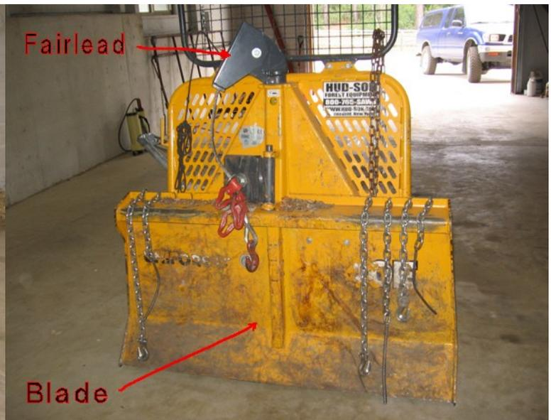
Skidding winches at the small end of the scale are usually driven by the tractor's PTO. Control ropes are used to engage the clutch and brake. The width of the 'blade' should be wide enough to extend from center line to center line of the back tires or more. This prevents logs from sliding up under the tractor and minimizes tire wear.
