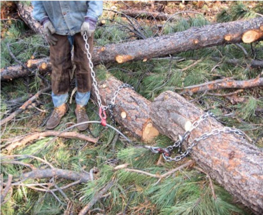
At left we have two chokers set, one on the end hook and one threaded through the slider. These two pieces are ready to be winched up to the blade.
