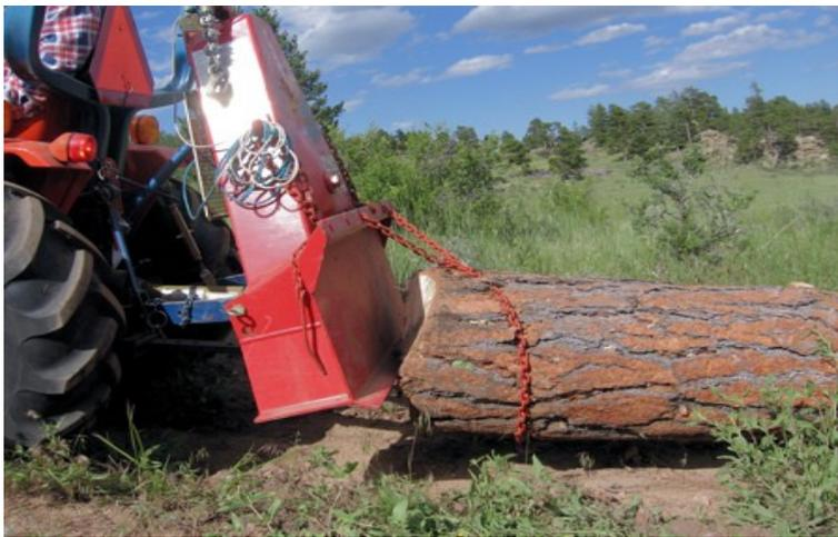
The log shown here is about the maximum weight that this equipment can skid while keeping the front end of the log off the ground. This is essential to minimize soil disturbance and rutting that can cause erosion.
