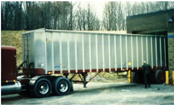
Mountain View School, Kingsley, Pennsylvania Facility Type: Two schools on adjacent properties System Size: 9.5 MMBH Manufacturer: Sylva Energy Systems Showing chip delivery from self-unloading tractor-trailer van.
