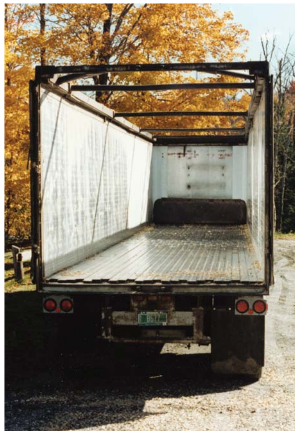
Trucks with a self-unloading or live bottom floor are often used to unload chips into a below-grade bin.
