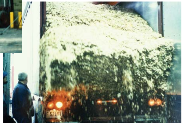
Mountain View School, Kingsley, Pennsylvania Facility Type: Two schools on adjacent properties System Size: 9.5 MMBH Manufacturer: Sylva Energy Systems Showing chip delivery from self-unloading tractor-trailer van.
