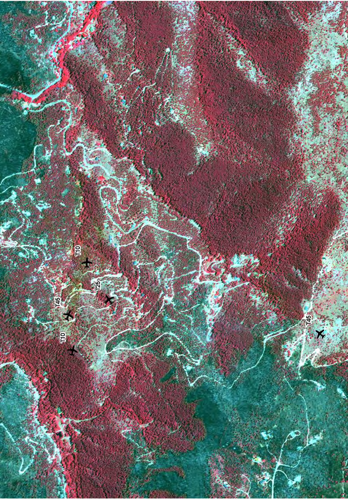
Figure 41. On September 8 several retardant drops were made in the Logan Mill Area . This area was under clouds in available satellite images for September 8, 2010. Background image displayed is a GeoEye-1 satellite image from September 10, 2010 at 11:42. Yellow paths in the image are retardant. A total of 5 drops were made in this area between 10:34 and 11:25.
