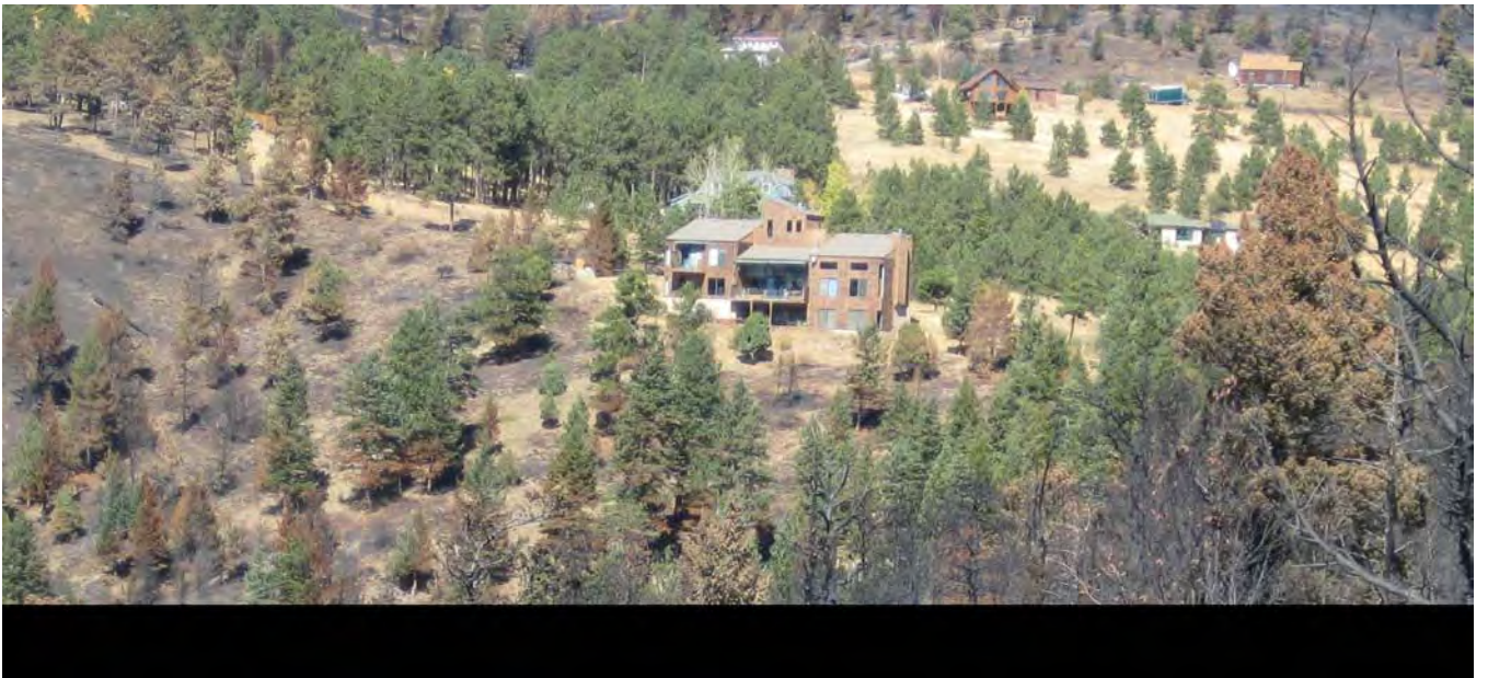
Figure 46. An example of homeowners treating both canopy and surface fuels around their home that resulted in low burn severity to the vegetation and the home survived a high intensity fire. Note the low burn severity resulting from a surface fire to the left of the home. Photos: Dan Steinman.
